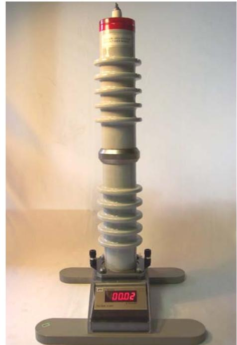
In single-phase test circuits, type TRV9940 is usually connected between the high voltage apparatus and ground, but the instrument can also be left “floating” if desired. With polyphase test circuits, type TRV9940 can be used to measure either line-ground or line-line voltages. Where the instrument is to be fully isolated (e.g. line-line measurements), our optional *insulating base assembly* is recommended (see OPTIONS below).
